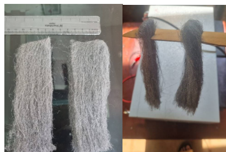
Fig. 3 Steel wool electrode and its orientation
